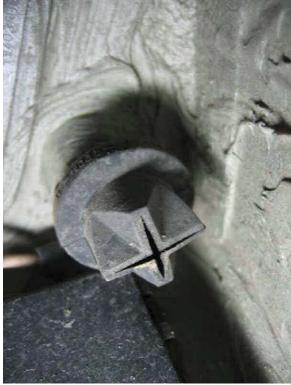
Whoever designed this should be shot or at least fired! The drain hole is about 8 mm in diameter, but the Internal tubing of the drain is only 5mm in diameter. Must get clogged eventually!!
