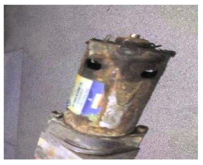
The repair is pretty difficult as the complete top needs to be removed to access the soft top motor (and we all know what can happen when your skilled dealer needs to do that kind of repair).
