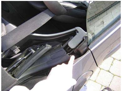
The drain on the left side is not visible because the soft top motor blocks the view. Now what happens: these drains get clogged, water can't get away and gets absorbed by the insulating foam. Result: soft top motor fails. (pic courtesy of www.zroadster.com !!!)
