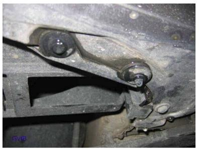
Make sure to unclip the ABS/DSC sensor that is clipped onto the splash thingy:
