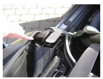
There is a water drain on each side. The drain on the right side (side of the fuel filler cap) is only visible if you watch closely between the soft top mechanism (top down) with a flashlight.
