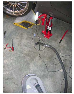
Same as on the right side, only here I didn't use compressed air, as the system is only accessible from the bottom. Instead, I modded my vacuum cleaner somewhat. A 6mm tube goes into 4mm tube... and that tube goes into the bottom of the drain:
